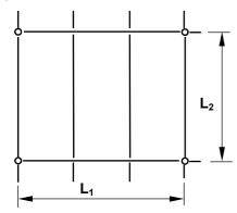
Floor number: C 7 D 8 Construction depth of the floor:  $H = b \cdot 4,2 m$ A ... L<sub>1</sub> = 7,5 m B ... L₁ = 9 m Laterally (2x) Longitudinally (6x)  $L_2 = a \cdot 7 m$  $v_{k} = c \cdot 4,0 \text{ kN/m}^{2}$ Operable load C ... S355J0+N D ... S235J2+AR Steel grade: Localization: permanent residence of student Terrain category: Α...Ι B ... II
