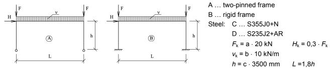
Design the structure for the highest possible utilization. Check the final design using the appropriate software (SCIA, Dlubal, etc.) and compare the results - explain the discrepancies.
